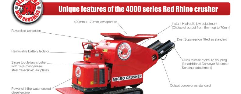
Description: Single toggle jaw crusher with jaw aperture of 400mm x 170mm - the only small crusher to accept a full UK kerbstone. The 4000 series is 775mm wide and can travel through doorways, into rear gardens, and enter sites where access and space is restricted. Hydraulically adjustable jaws allow for the adjustment of output product size, ranging from a choice of 5mm up to 70mm.
